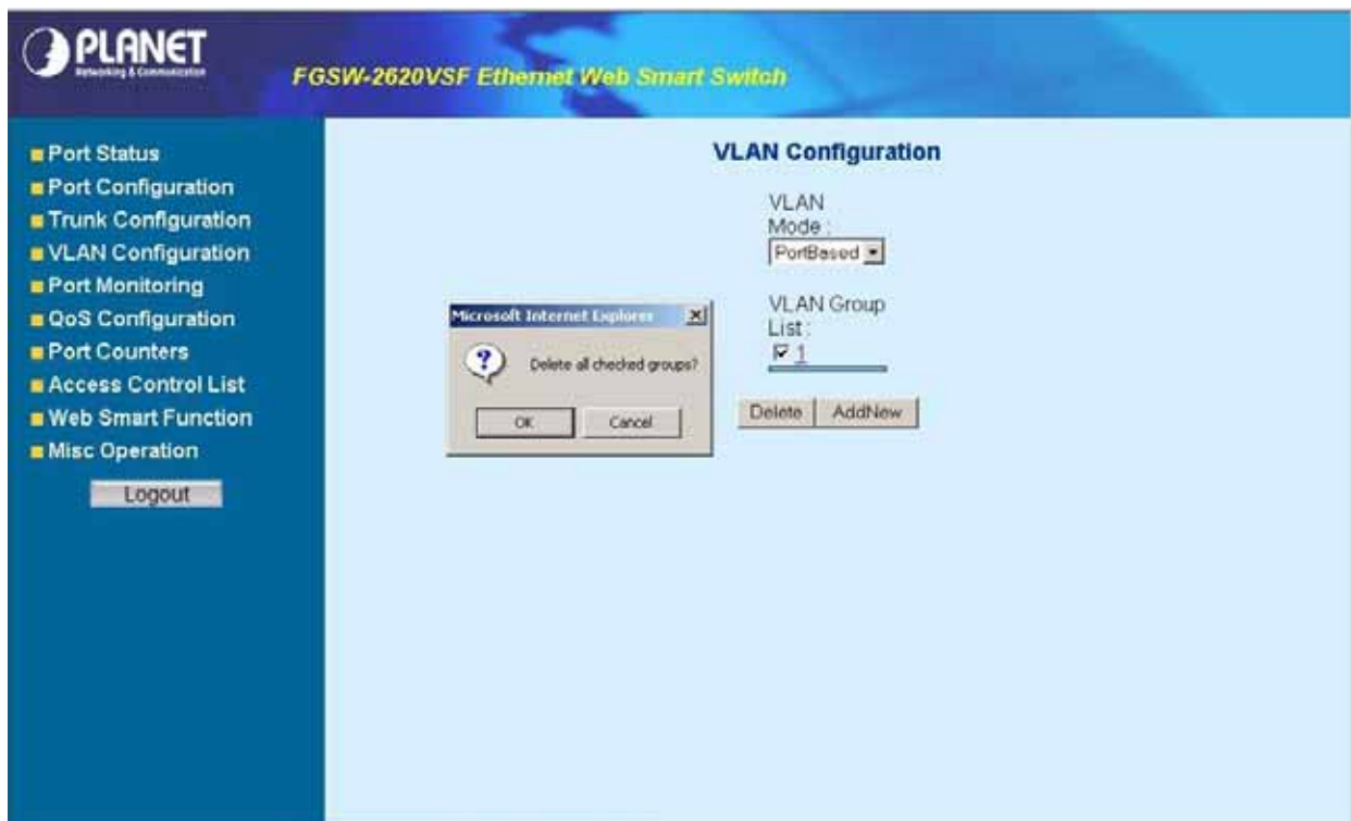
Figure 4-20 Delete Port-based VLAN group Web Page screen
